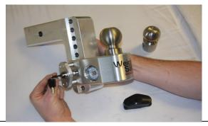
**STEP 3:** Insert the <u>Keylock Assembly (WS03)</u> into the <u>Weigh Safe Slider</u> when you have achieved the desired position along the Drawbar and lock in place by turning
