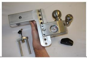
**STEP 1:** Ensure that the <u>Ball Retaining Pin</u> is inserted fully into the <u>Weigh Safe slider</u>. Do not operate without ball pin in place.
