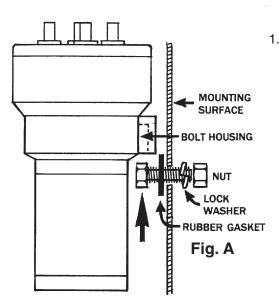
Install the compressor in the engine compartment in a dry location and safe from engine exhaust manifold heat. To secure the compressor, drill a 3/16-inch hole through metal and mount compressor vertically (air outlets at the top). Insert head of bolt into the bolt housing and secure to the vehicle referring to Figure A. Use mounting hardward in the order shown – bolt, rubber gasket, mounting surface, lock washer, nut.
