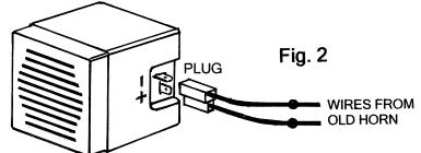
11. Connect the plug to the EE100. The horn installation is complete and the horn is ready to be used.
