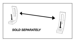
Insert the supplied bolts into the rear of the SAR Light bar. These will slide in on the side nearest the orientation button as shown in the first diagram to the right. Insert the rubber spacers onto the bolts. Position the light bar near the brackets, insert the bolts into the brackets, and secure with the included nuts and lock washers. To adjust rotation or to move the light bar from left to right, simply loosen these nuts, reposition, and snug back.
