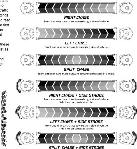
Front and rear bars chase outward towards both sides of vehicle. Side bars on constant strobe.
