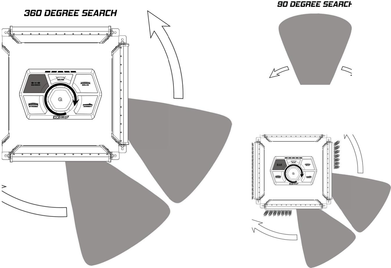
Search Mode allows the user to direct the light where necessary. To activate Search, simply click the Search button. The forward-facing light bars will illuminate and can be controlled via the center turn dial. Turn the dial clockwise to direct right, and counterclockwise to direct left.
