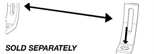
Insert the supplied bolts into the rear of the SAR Light bar. These will slide in on the side nearest the orientation button as shown in the first diagram to the right. Insert the rubber spacers onto the bolts. Position the light bar near the brackets, insert the bolts into the brackets, and secure with the included nuts and lock washers. To adjust rotation or to move the light bar from left to right, simply loosen these nuts, reposition, and snug back.
