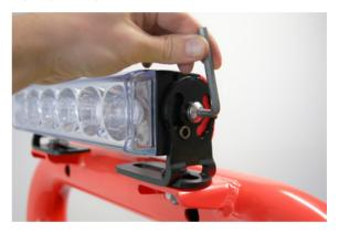
Once driving light up/down alignment is completed, fully tighten the centre bolts on each end using 6mm Allen key
