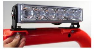
Position driving light in desired mounting location, then loosely fix main mounting bolt washers and nuts to hold the light into position (do not tighten at this stage as mounting bolts need to be left loose until final alignment adjustments have been made at the end of the installation process)
