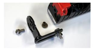
Identify the mounting bracket that contains the adjustment device, remove centre bolt and mounting foot, while taking care not to lose the adjustment cam
