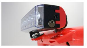
Then re-insert the adjustment cam on the adjustment end of the driving light (hex socket at top), remove the nut and washers from the main mounting bolt (leave the bolt itself and off-centre cam in place), then place mounting foot into required position—selecting suitable hole in the mounting bracket for the adjustment cam (plus reverse mounting foot 180° if outward position is required), and loosely reinstall the centre bolt
