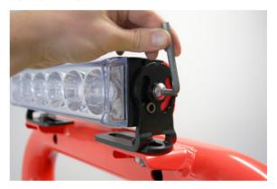
Once driving light up/down alignment is completed, fully tighten the centre bolts on each end using 6mm Allen key
