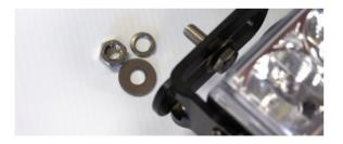
• Remove the nut and washers from both main mounting bolts, but leave both bolts and off-centre cams in place
