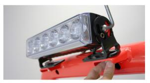
• Then loosely fix main mounting bolt washers and nuts to hold the light into position (do not tighten at this stage as mounting bolts need to be left loose until final alignment adjustments have been made at the end of the installation process)
