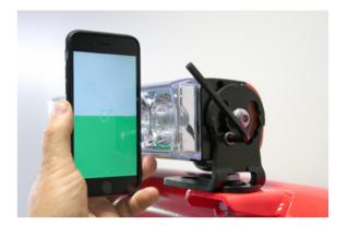
For up/down alignment, use a 6mm Allen key to turn the adjustment cam up or down until you reach the desired beam angle of 0° (90° to the horizontal plane); many modern smartphones have a leveling App built-in
