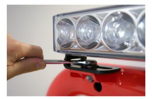
For left/right beam alignment, use a 17mm spanner and rotate the bolt head left or right until the desired alignment is acheived; note: approximately 6mm of forward and backward adjustment is available on each side
