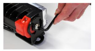
Using a 6mm Allen key, loosen centre bolt on the non-adjustment end (to reverse mounting foot to outward position, fully remove centre bolt, turn mounting foot 180°, refit centre mounting bolt without tightening)
