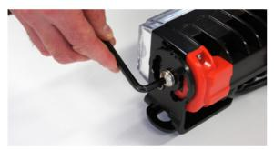
Using a 6mm Allen key, loosen centre bolt on both ends, but do not remove
