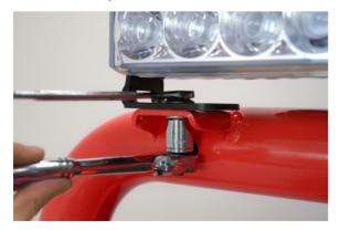
Once satisfied with the left/right alignment, hold a 17mm spanner in place on bolt head (to maintain alignment position) and use a 17mm socket to tighten the nuts on the underside of the main mounting foot bolts
