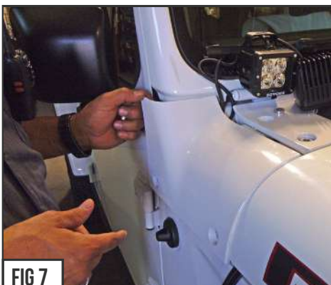
INSTALLERS NOTE: Mock Up LED Lights and plumb wires.
