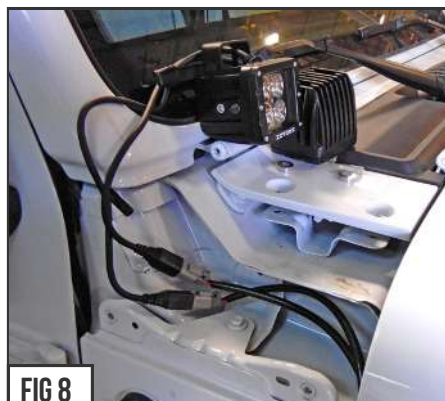
INSTALLERS NOTE: Mock Up LED Lights and plumb wires.
